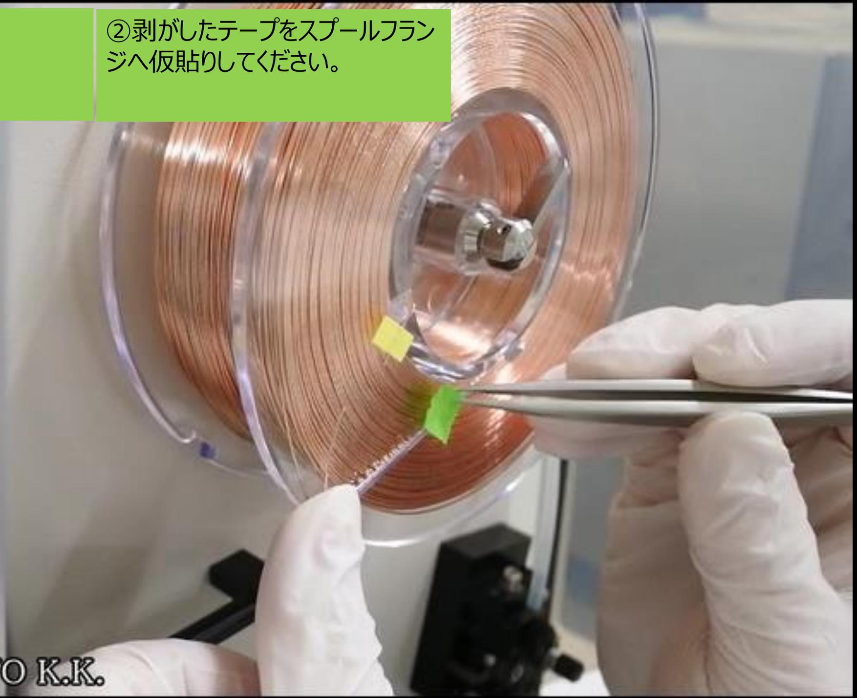
②Attach the peeled tape temporarily to the flange.
