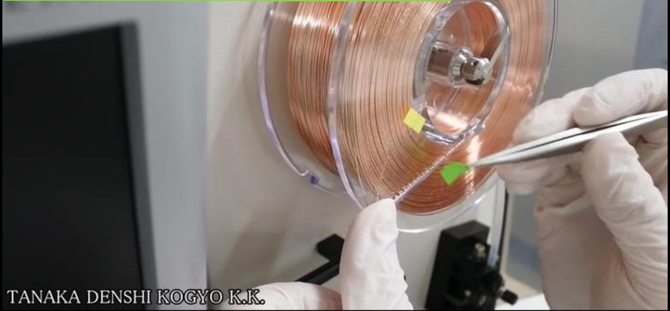
②Attach the peeled tape temporarily to the flange.
