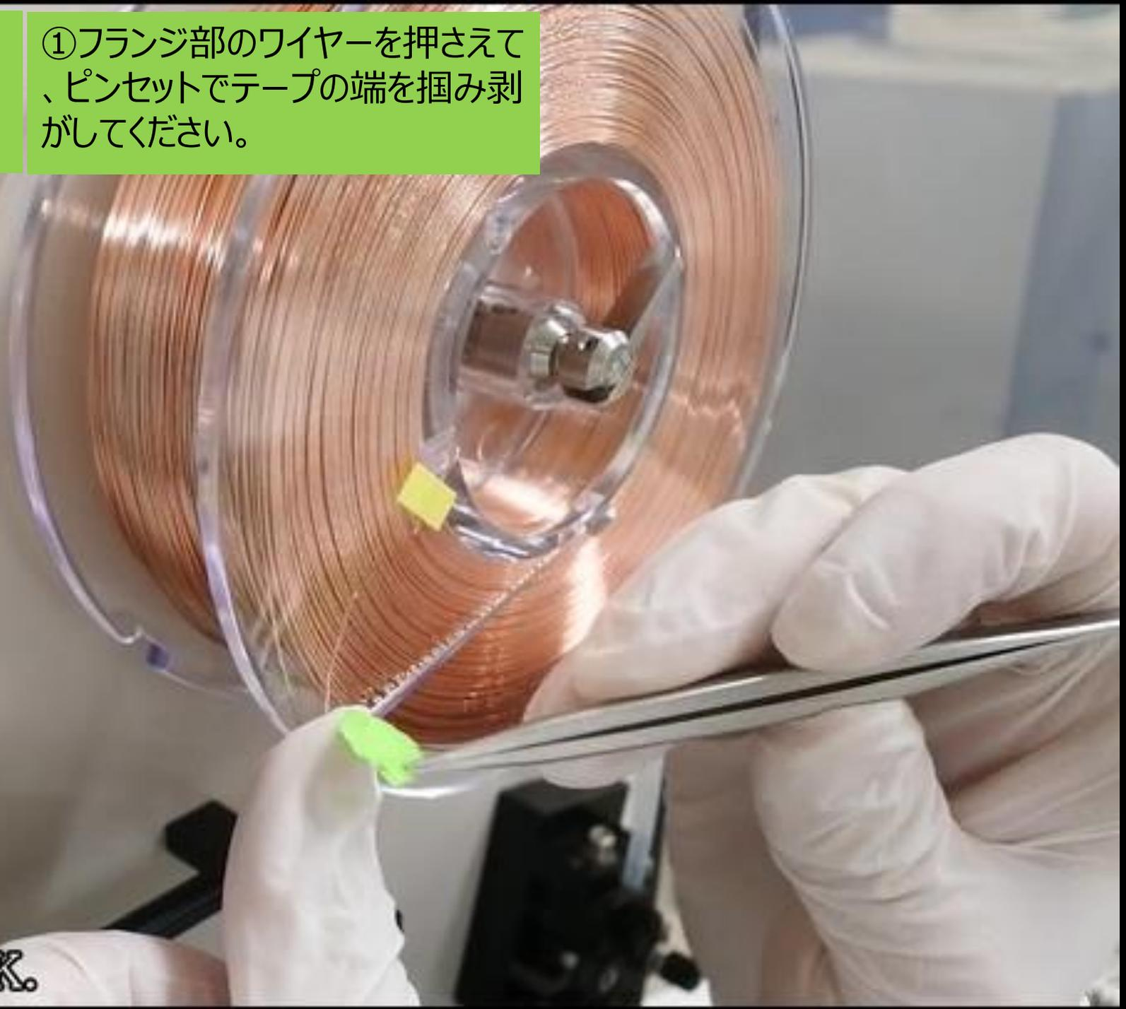
① Hold the wire on the flange, pinch the edge of the tape with tweezers and peel it off.
