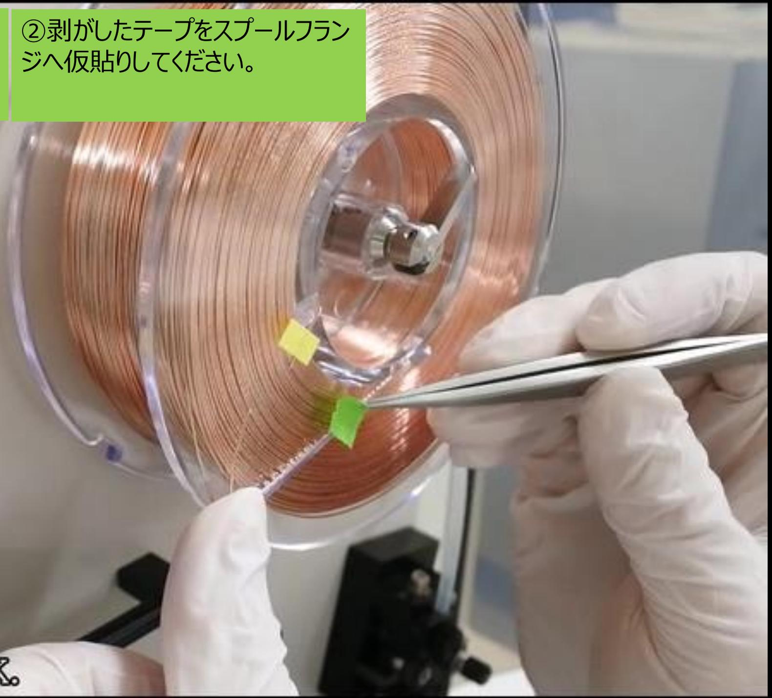
②Attach the peeled tape temporarily to the flange.
