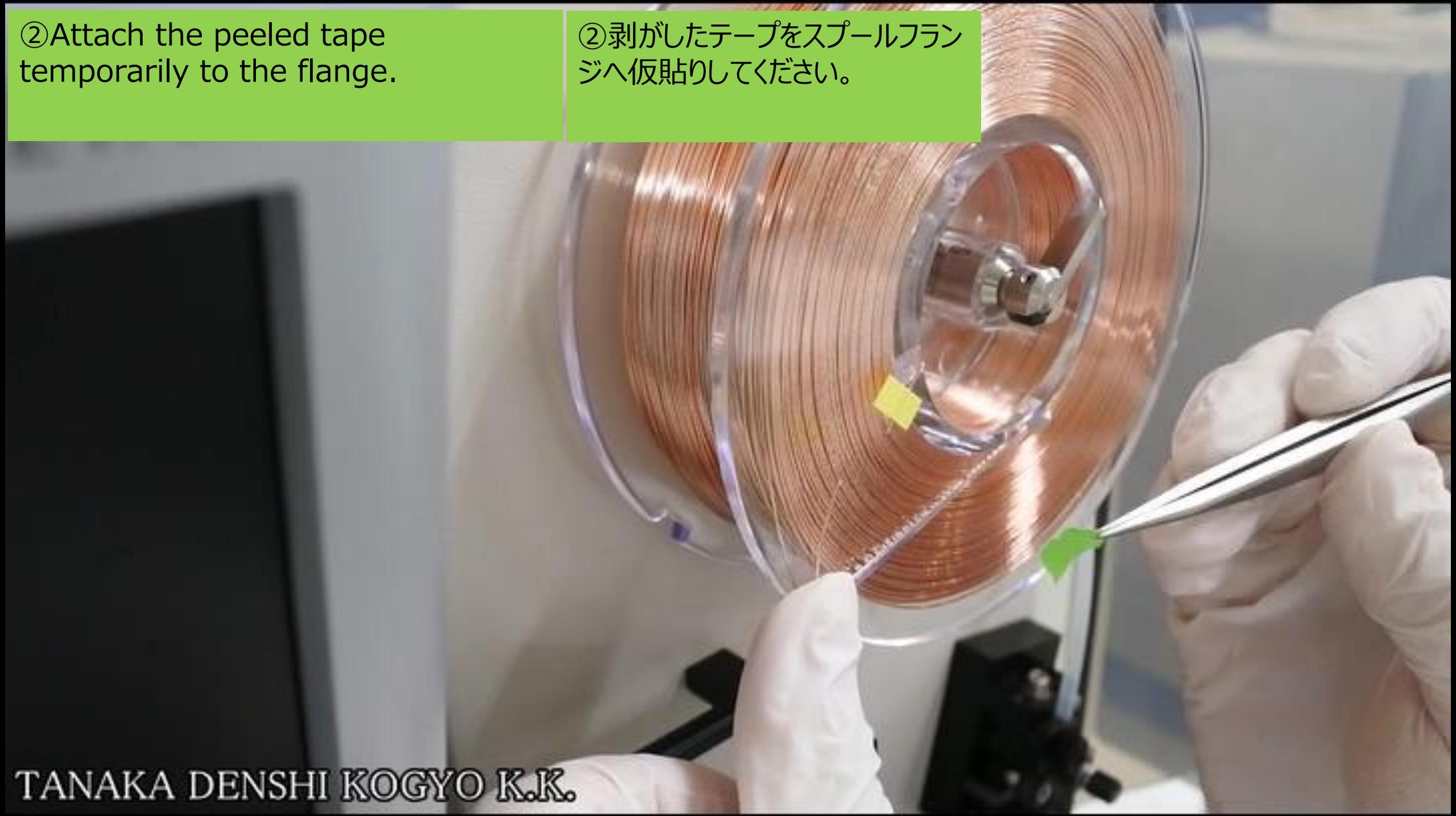
②Attach the peeled tape temporarily to the flange.
