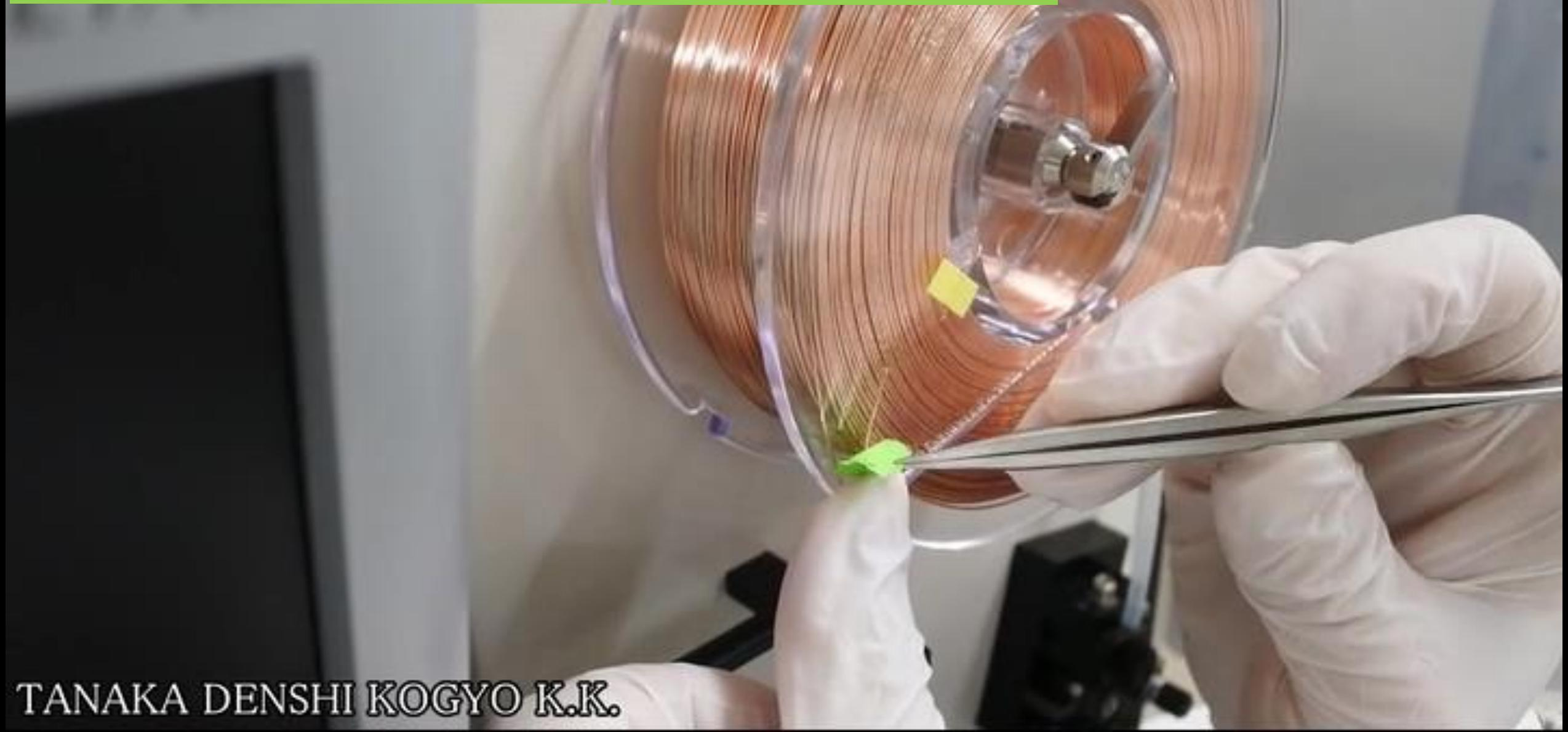
① Hold the wire on the flange, pinch the edge of the tape with tweezers and peel it off.
