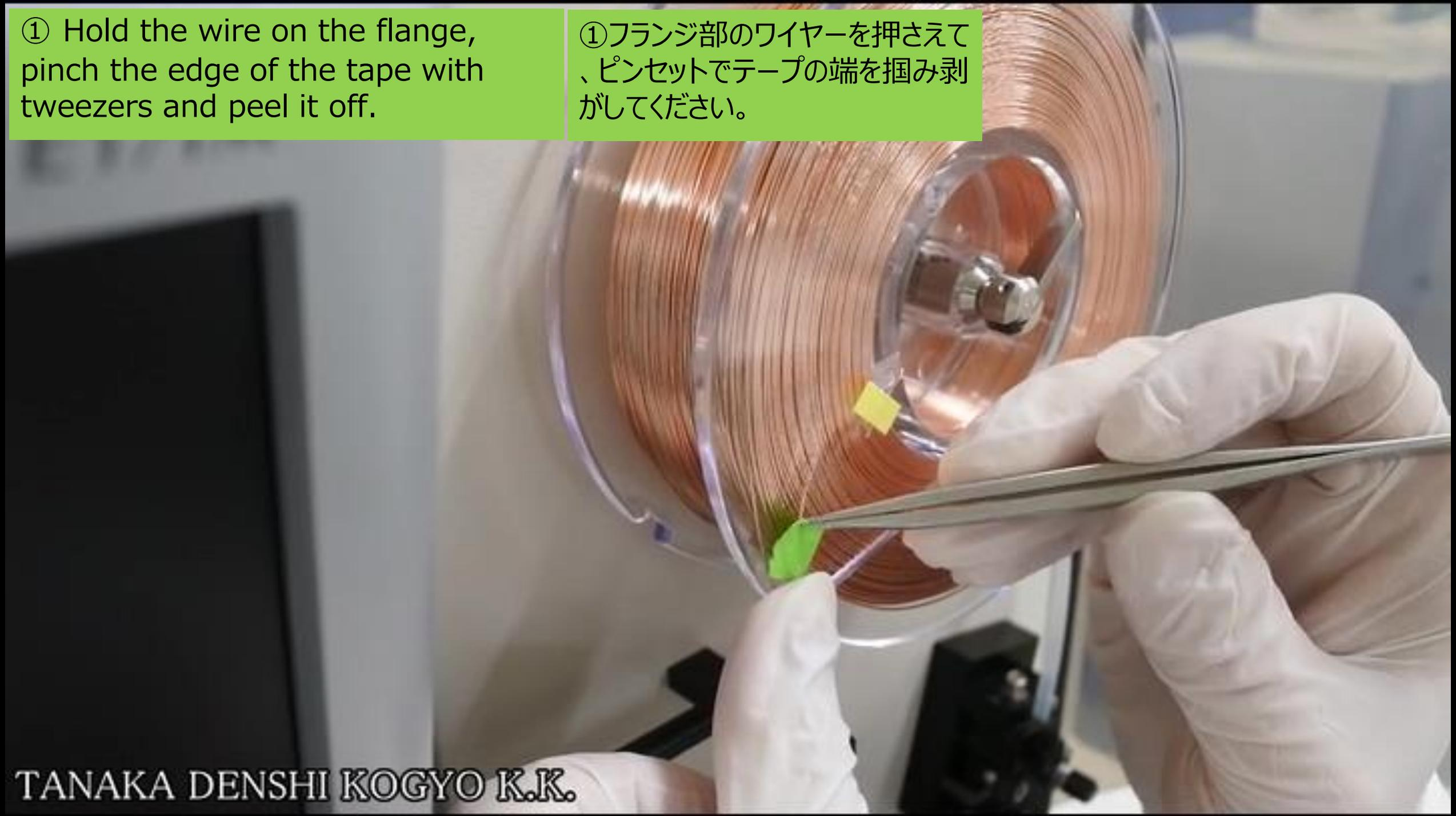
① Hold the wire on the flange, pinch the edge of the tape with tweezers and peel it off.
