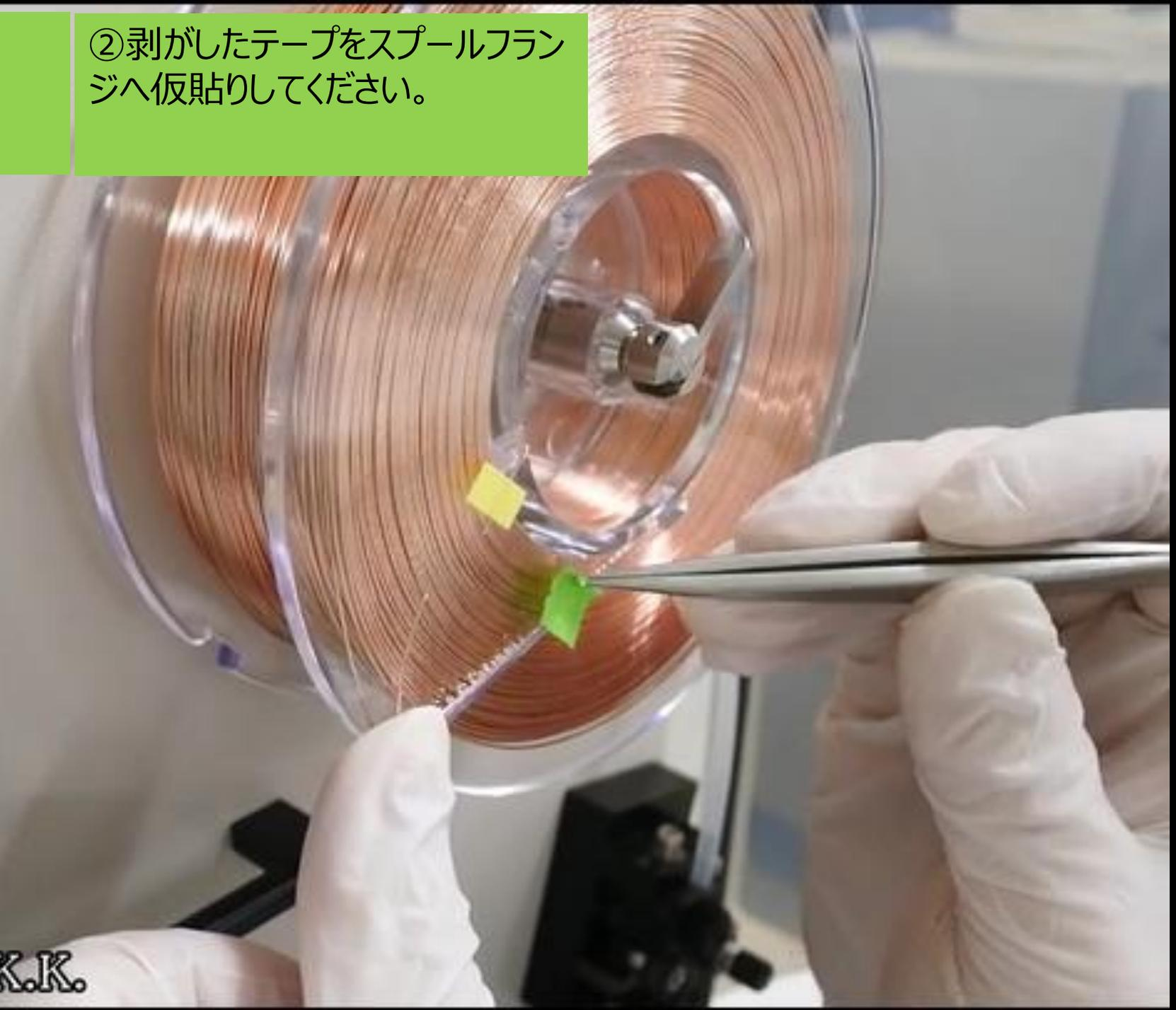
②Attach the peeled tape temporarily to the flange.
